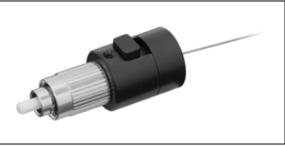
Click for Exploded View The BFTU terminator secures the connector using a 2-56 setscrew and the fiber using a spring-loaded button-actuated clamp.
